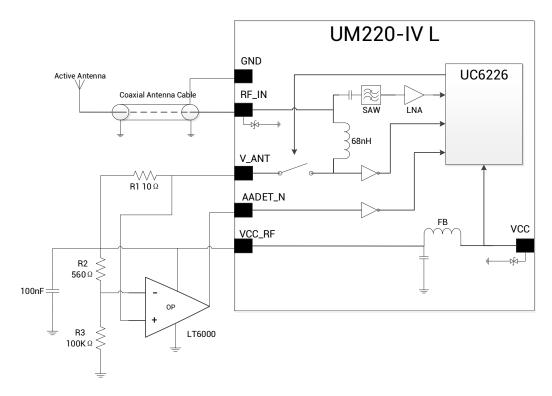
Figure 3-1 Reference Circuit of Antenna State Detection
