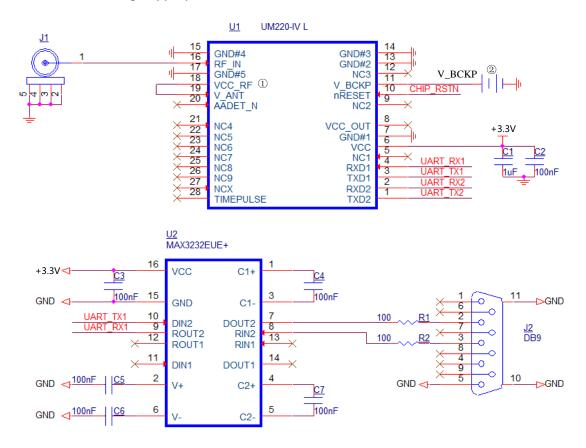
Figure 1-1 Minimum System Reference Circuit
